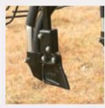
25mm coil tines with Duncan 'T' boot and a tungsten tile on the leading edge giving accurate seeding with superior strength and wear
